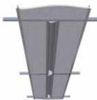
Recommended distance from fixture longitudinal axis and wall is 1' to 3'. Optimum performance distance is 2'. Not recommended for use outside this range. Fixture housing lengths are 3', 4' and 5' mounted individually in grid ceilings and in sheet rock. Can be mounted in continuous rows.
